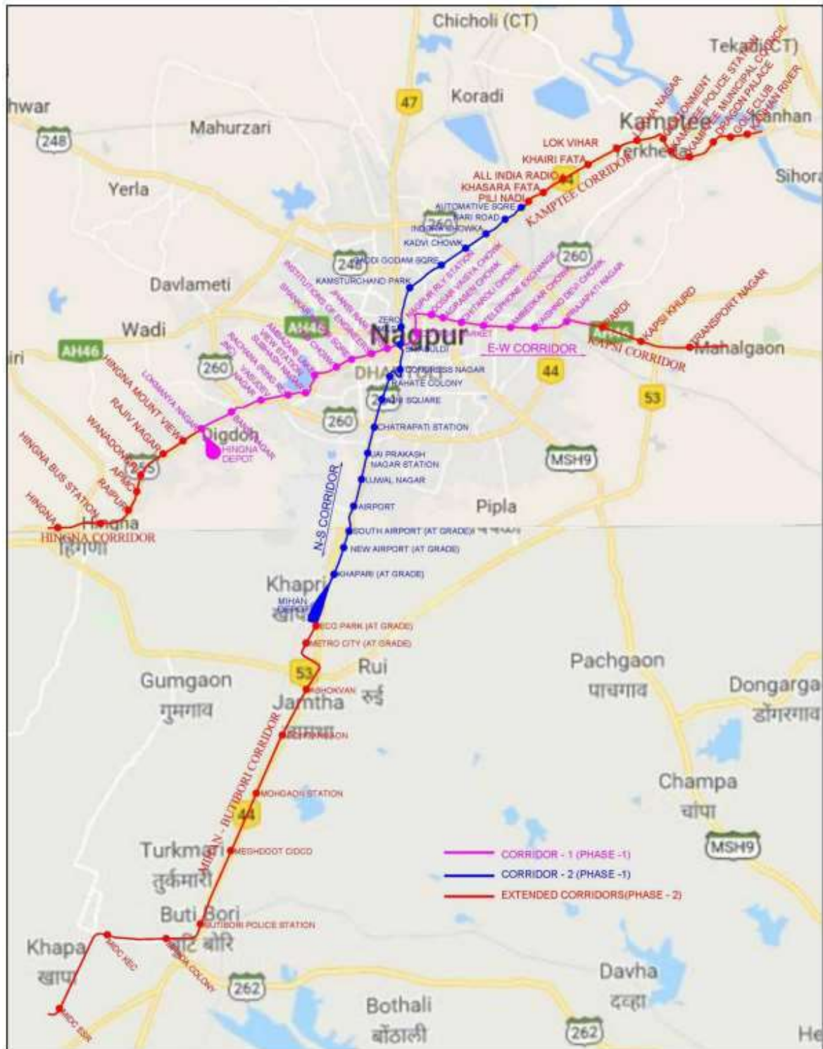
Figure 1: Routes of NMRP Phase II
